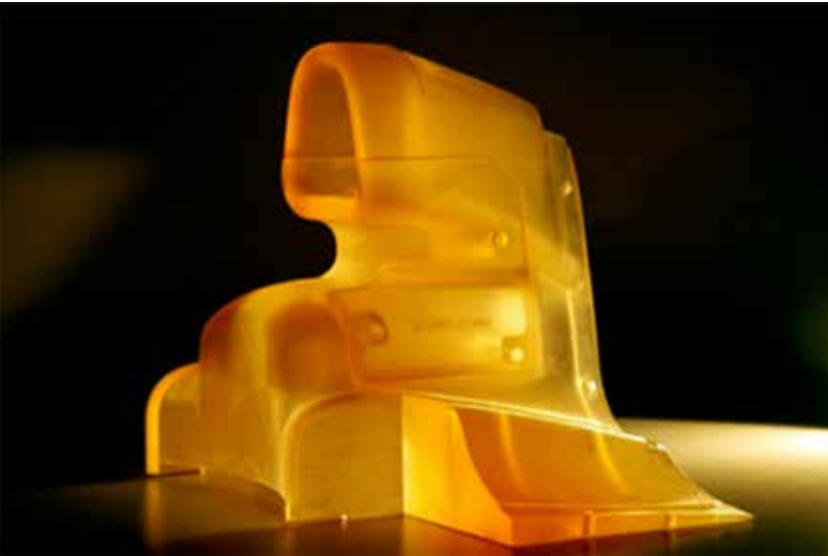
IMG.2 (Wind Tunnel model SLA Air-box)
