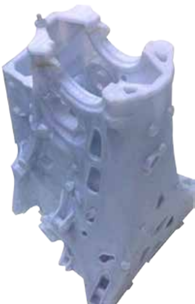
IMG. 4 Gearbox casting pattern
